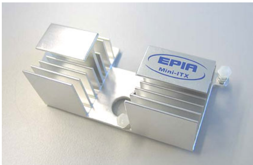
Chipset-heat sink of VIA M10000
